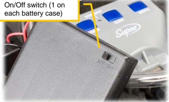
On/Off switch (1 on each battery case)
