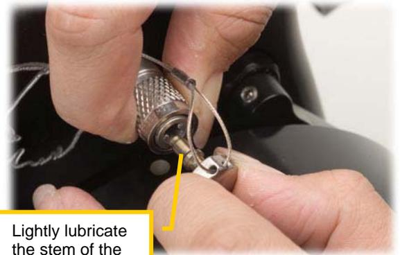
Lightly lubricate the stem of the stem plug
